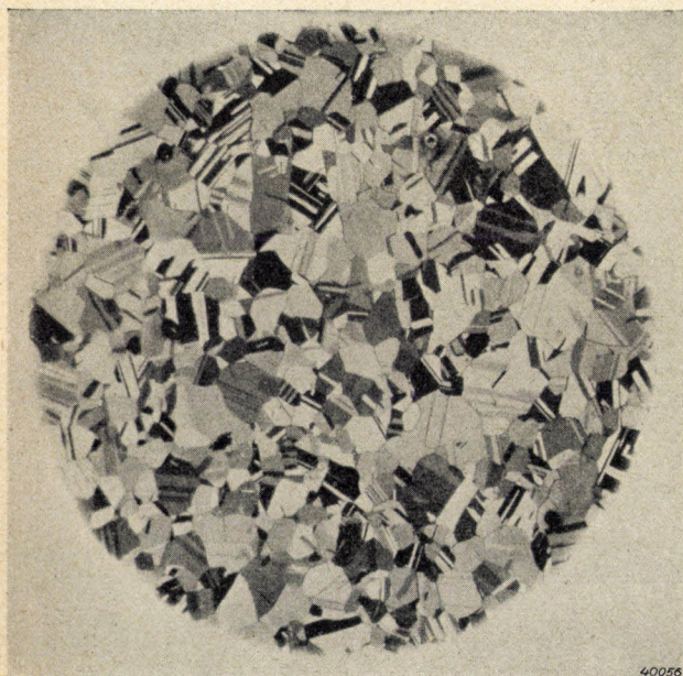
Fig. 1. Photomicrograph of polished and etched \alpha -brass (magnified 100 times). The polycrystalline structure is here clearly visible because of the fact that the different crystal grains reflect the light in different ways.
