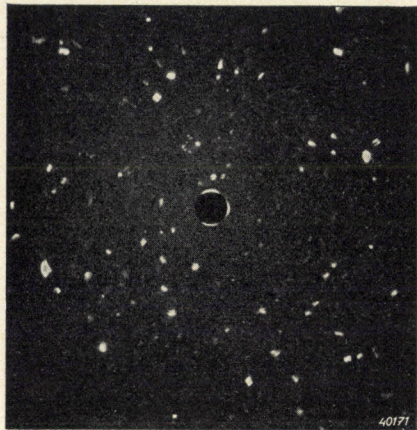
Fig. 6. Laué photograph of cross-rolled molybdenum which was afterwards annealed at 1300^{\circ}\text{C} . The texture has disappeared entirely. (Laué photographs are made with X-radiation having a continuous spectrum. This is necessary in this case since with monochromatic radiation the few randomly oriented crystal grains present will not in general satisfy Bragg's equation, so that no reflections at all will be obtained. With a continuous spectrum on the other hand there is for every lattice plane in every grain a ray with a wavelength which can be reflected).
