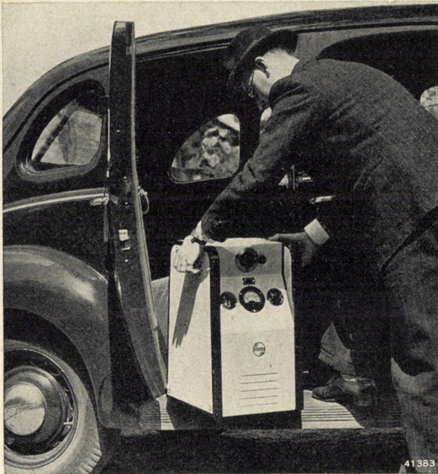
Fig. 4. Generator for short-wave therapy, type 11 951. The apparatus weighs only 28 kg and can easily be transported in a motor-car. The maximum effective high-frequency output amounts to 150 W.
