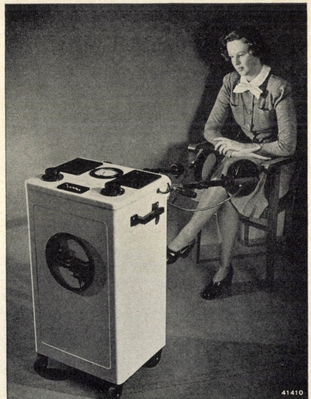
Fig. 3. Generator for short-wave therapy, type 11 952, in use (treatment of knee joint). This apparatus in the form of a desk on wheels can deliver a maximum high-frequency output (wavelength 5 m) to the patient. Besides the knob for switching on (right) there is no other part to be operated by the medical personnel but the knob for adjusting the desired output (left), which is read off on the meter, and the disc for tuning the circuit with the patient (centre), which is checked on the same meter. Dimensions 46 × 37 × 87 cm, weight 62.5 kg. Two electrodes in the form of plates are fastened to the apparatus by means of two arms which can be turned in all directions.
