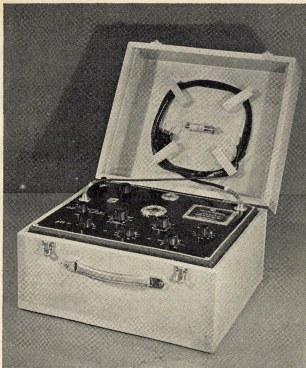
Fig. 11. The apparatus is built into a metal box which is made moisture tight. An opening covered by a magnifying lens for the cathode ray indicator may be seen. Above it is a second window giving access to a quantity of silica gel as drying agent. By using a strong baked lacquer, by chromium plating certain parts and by making it very tight against moisture, every attempt has been made to make the instrument suitable for use in chemical laboratories. Further protection is given by a heavy wooden case.
